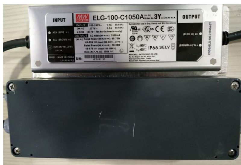
5) LED driver and connection box
