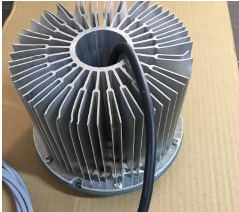
8) Internal wiring where it enters to cooling fin and connected to LED module
