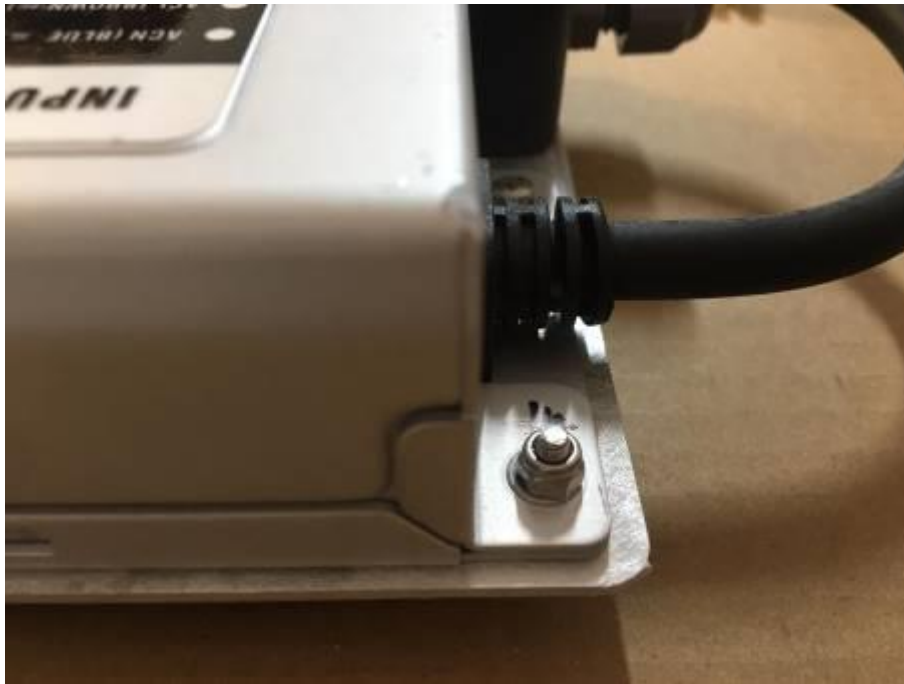
10) Earthing connection for LED driver enclosure
